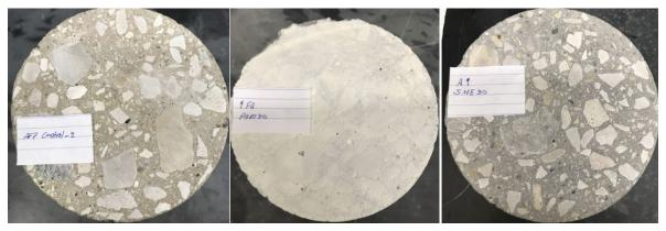
(a) Control (b) PAM-coated Sample (c) SME-PS Sample Figure 4.2 Samples for Chloride Diffusion Testing
