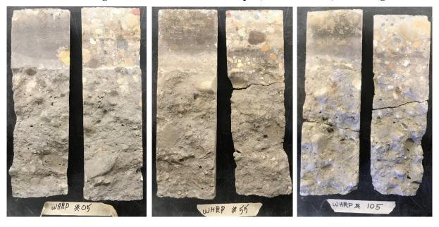
Figure F.2 I-39 Silane-Treated Core Samples, as-received left, cleaned right
