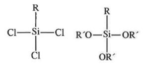
R is the organofunctional group; OR' is the silicon functional group Figure 2.2 (a) chlorosilane (b) silane and siloxane
