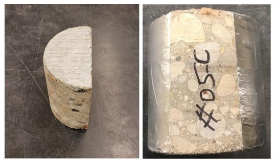
Figure F.6 Preparation of Core Samples for Absorption Testing, epoxy-coating surface (left) and aluminum tape on shoulders and exposed top (right)
