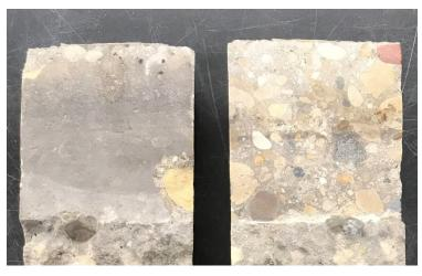
Figure 5.7 Silane-treated core sample (left) as received and (right) after cleaning
