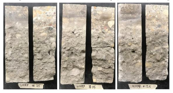
Figure F.4 I-39 SME-PS Treated Core Samples, as-received left, cleaned right
