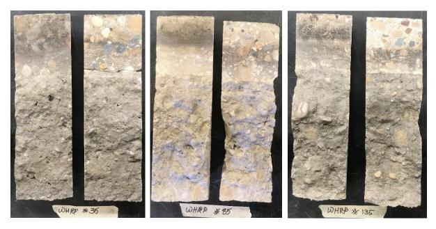
Figure F.5 I-39 Lithium Silicate Mixture-Treated Core Samples, as-received left, cleaned right
