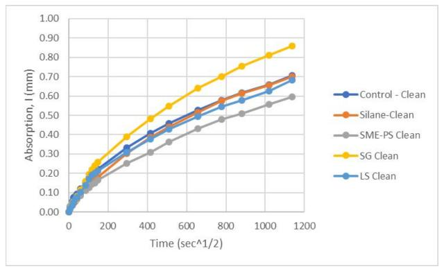
Figure F.12 I-39 Average Clean Core Absorption
