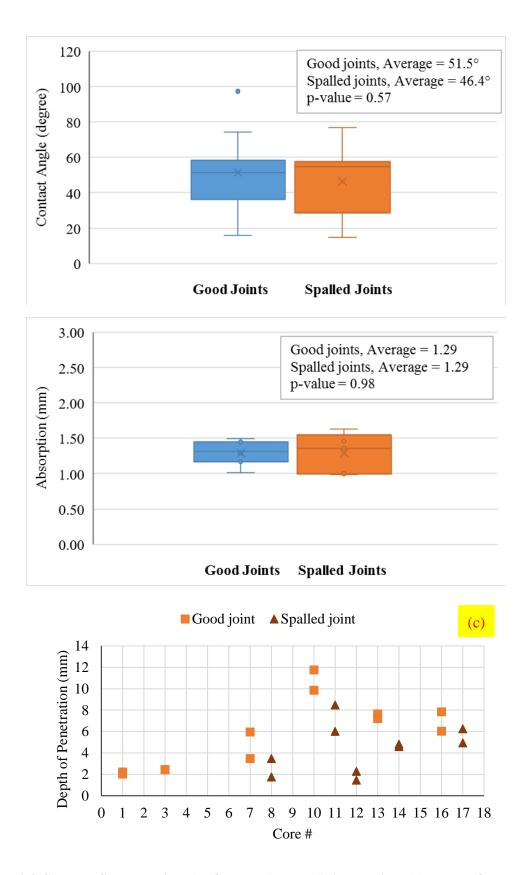
Figure 3.8 Good vs. Spalled Joints (a) Contact Angle, (b) Absorption, (c) Depth of Penetration
