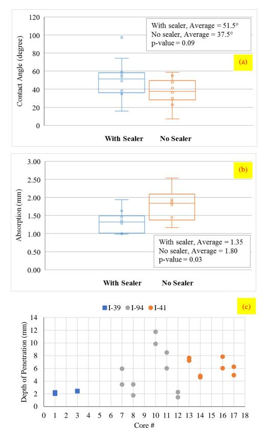
Figure 3.6 Presence of Sealer (a) Contact Angle, (b) Absorption, (c) Depth of Penetration
