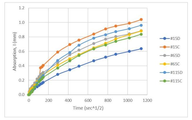
Figure F.10 I-39 Siloxane Mixture-Treated Core Absorption
