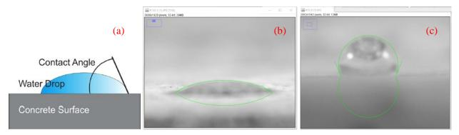
Figure 3.3 (a) Definition of contact angle (b) Contact angle=32.5° for core #135 (c) Contact angle =112.5° for core #15
