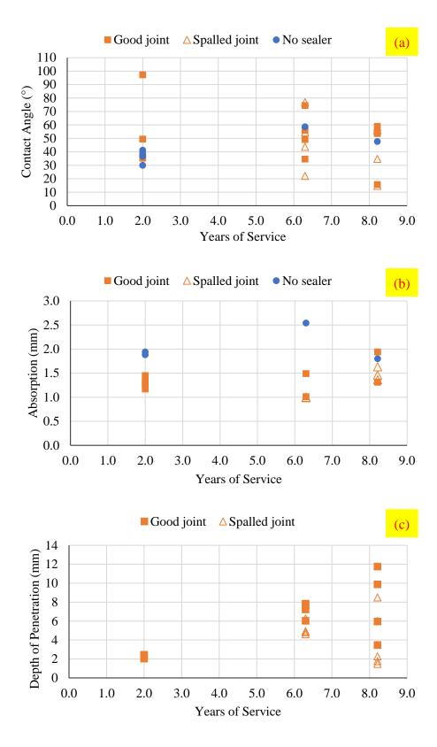
Figure 3.7 Service Life (a) Contact Angle, (b) Absorption, (c) Depth of Penetration
