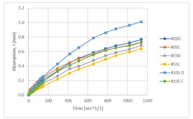
Figure F.8 I-39 Silane-Treated Core Absorption
