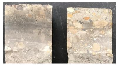
Figure 5.6 Untreated core samples (left) as received and (right) after cleaning
