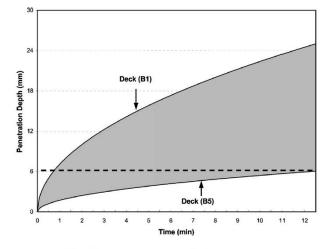
Fig. 4. Silane penetration depth against time
