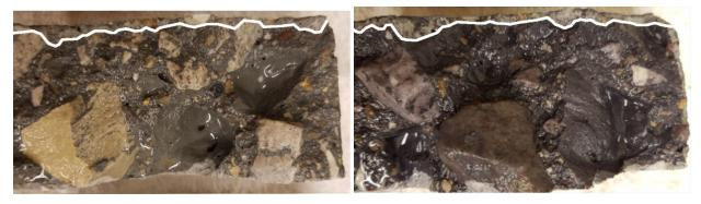
Figure 4.4 Example Depth of Penetration for SME-PS Specimen (Left: water, Right: blue fabric dye)
