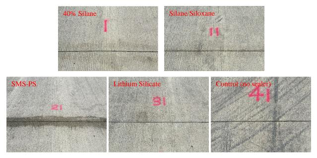
Figure 5.2 Appearance of Joints Right After Sealer Applied
