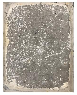
Figure C.5 FA Silane applied dry after 50 Cycles
