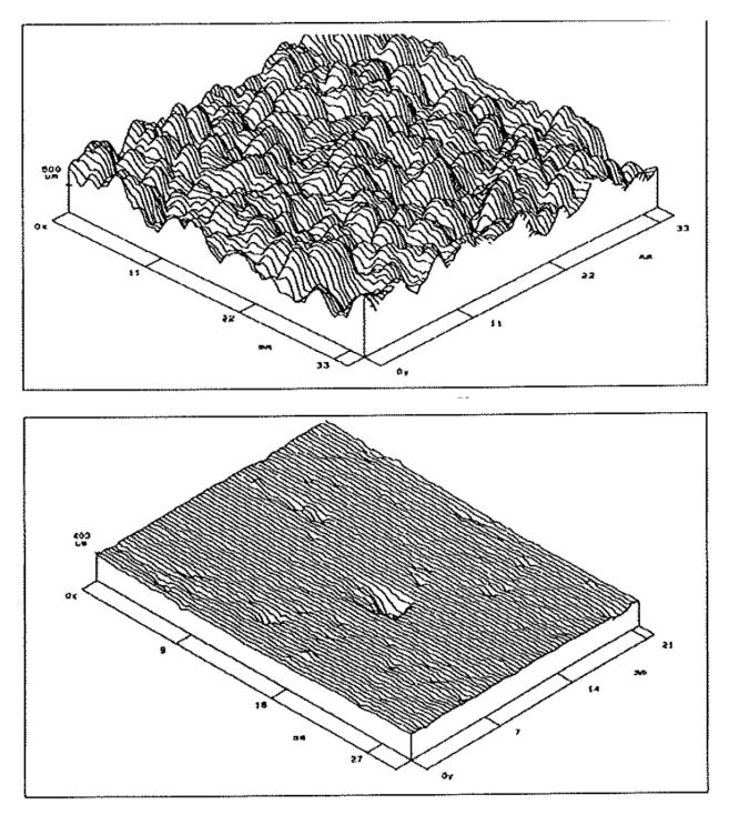
Figure 5.8 3D visualization of (a) sandblasted and (b) polished concrete profile (Courard, 2000)
