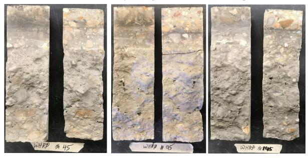
Figure F.1 I-39 Control Core Samples, as-received left, cleaned right
