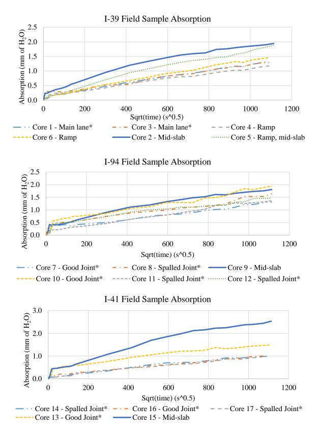
Figure A.1 Absorption of Core Samples from I-94, I-41, and I-39
