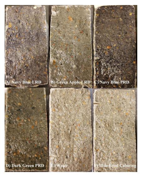
Figure C.3 Secondary Dye Testing for Depth of Penetration
