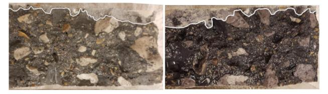
Figure 4.3 Example Depth of Penetration for Silane Treated Specimens (Left: water, Right: blue fabric dye)
