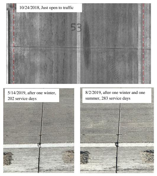
Figure 5.3 Field Performance of Joint #53
