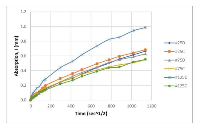
Figure F.9 I-39 SME-PS-Treated Core Absorption
